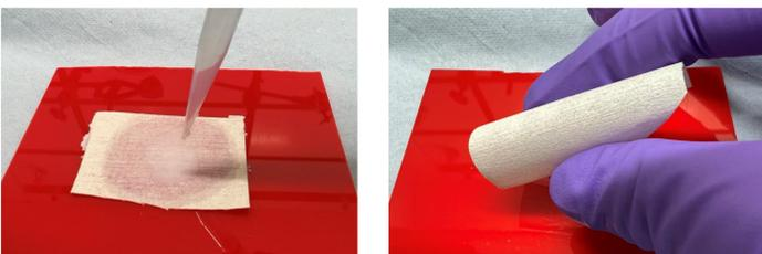
Figure 5: Left - h-BN/polymer ink was drop casted on a textile; Right - flexibility of the textile after being coated.
