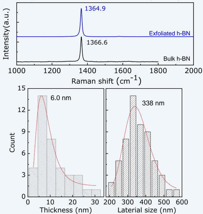
Figure 3: Raman (top) and AFM (bottom) characterization of exfoliated h-BN flakes.
