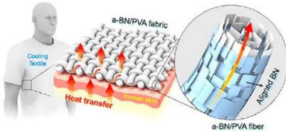
Figure 1: Structure illustration of a designed cooling textile, image reproduced from REF [1].
