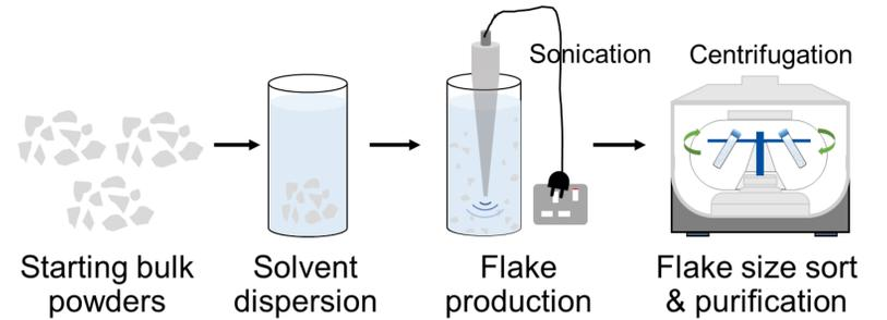
Figure 2: Step-by-step ultrasonication-assisted liquid phase exfoliation.
