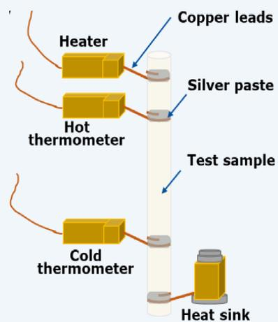
Figure 4: Left - illustration of the thermal experimental setup; Right - thermal conductivities of the composites with varying mass fractions of h-BN.
